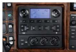
HAVC System Combine Controller (Convenient Interior Air conditioning · Heating Control)
