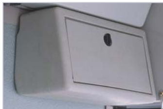
Driver console box
